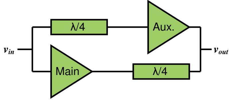
Figure 1.4 Block diagram of a Doherty PA.
