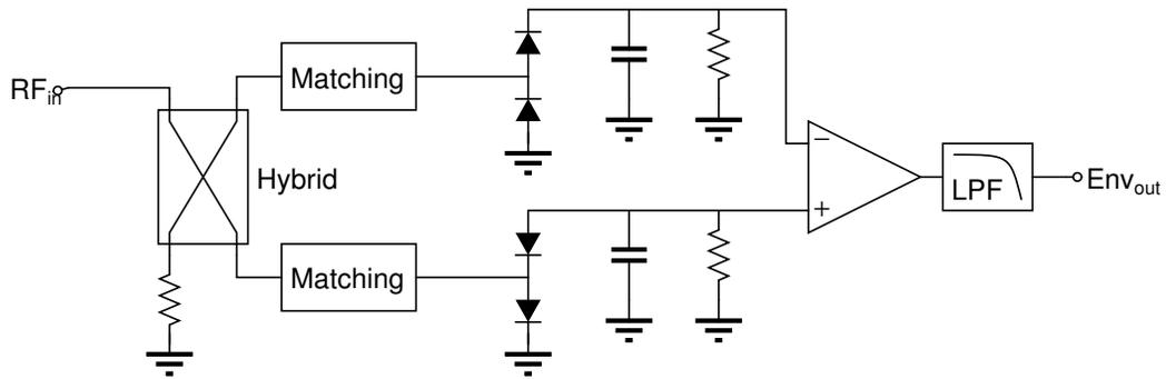
Figure 3.11 Circuit implementation of the envelope detector.
