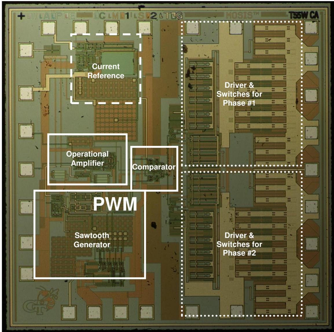
Figure 4.10 Die photo of dual-phase PWM supply circuit.
