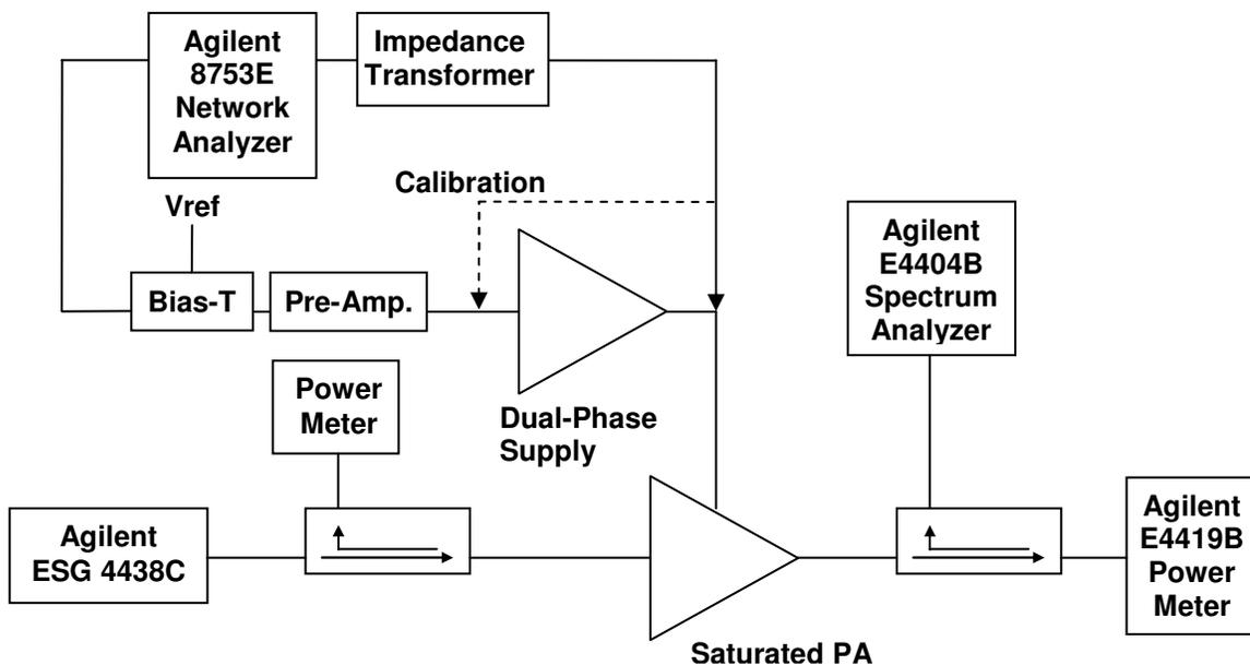
Figure 4.16 Measurement setup for frequency response characterization.
