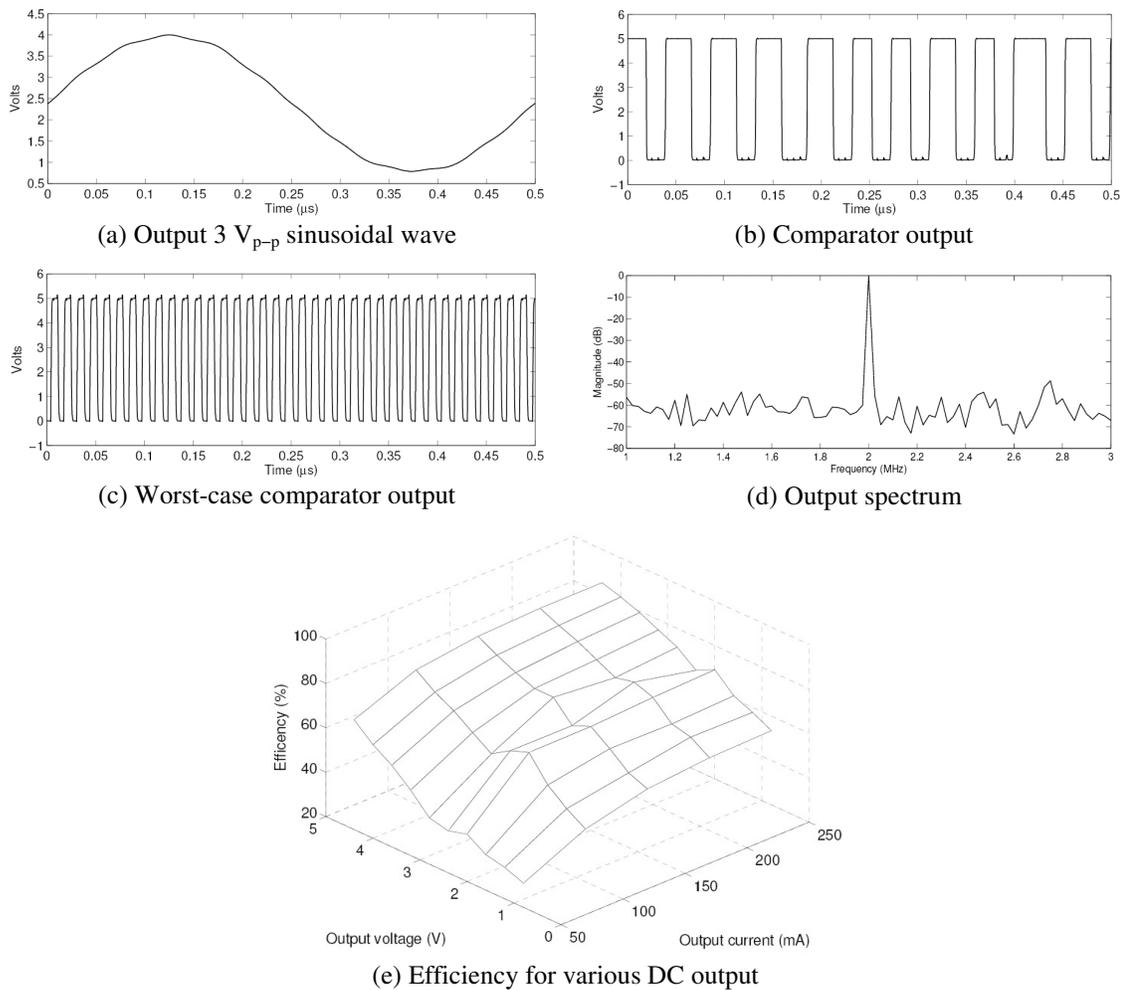
Figure 3.7 Simulation results of delta-modulated dynamic supply circuit.
