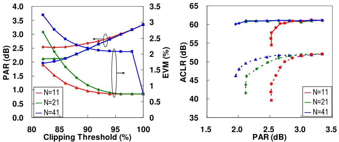
Figure 4.33 System-level simulation of CFR using subtraction of Kaiser-windowed sinc function with various filter lengths for W-CDMA.
