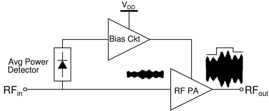
Figure 2.5 Block diagram of a power-level tracking PA.
