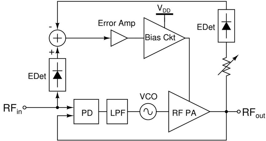
Figure 2.6 Block diagram of a polar modulated PA.
