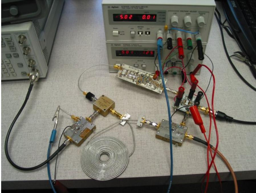
Figure 3.12 Measurement setup for CDMA EER PA.
