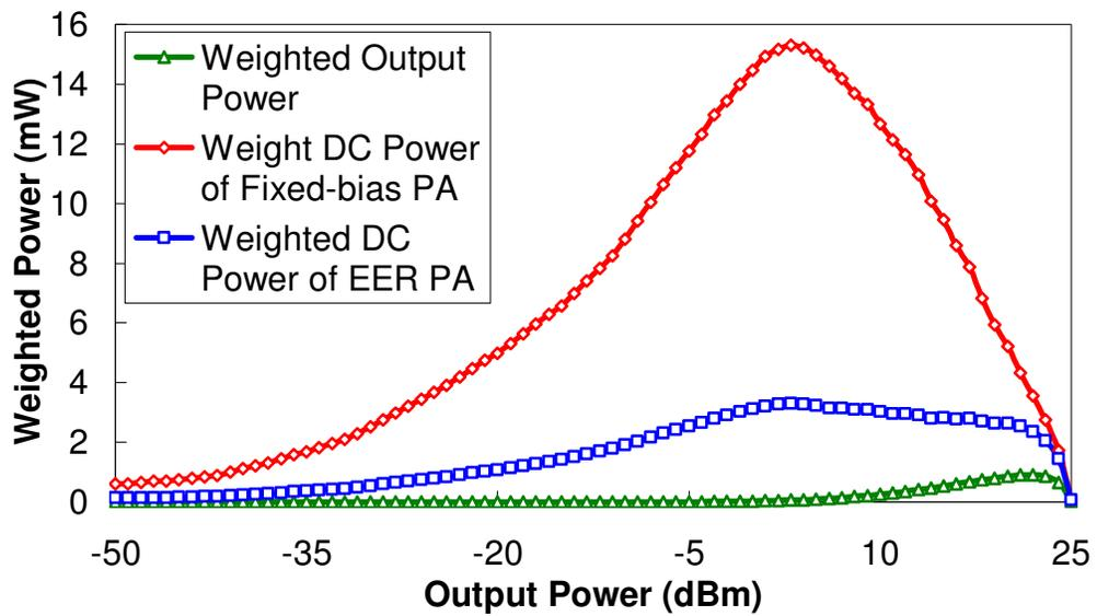
Figure 3.15 Comparison of weighted power using urban area probability distribution function.
