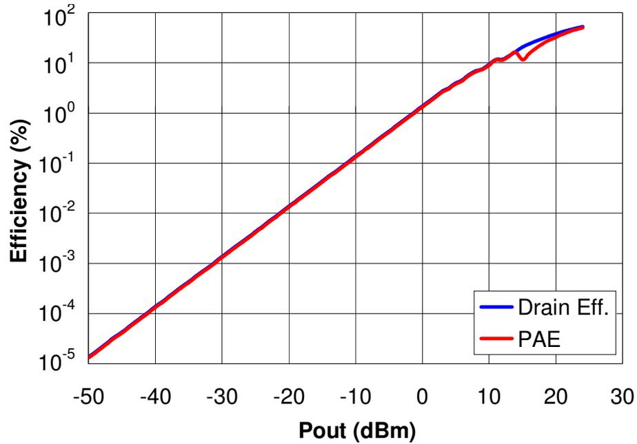
Figure 4.43 Drain efficiency and PAE comparison of dual-mode PA using EER technique for  $P_{out}$  greater than 14 dBm and PT technique for lower output power.
