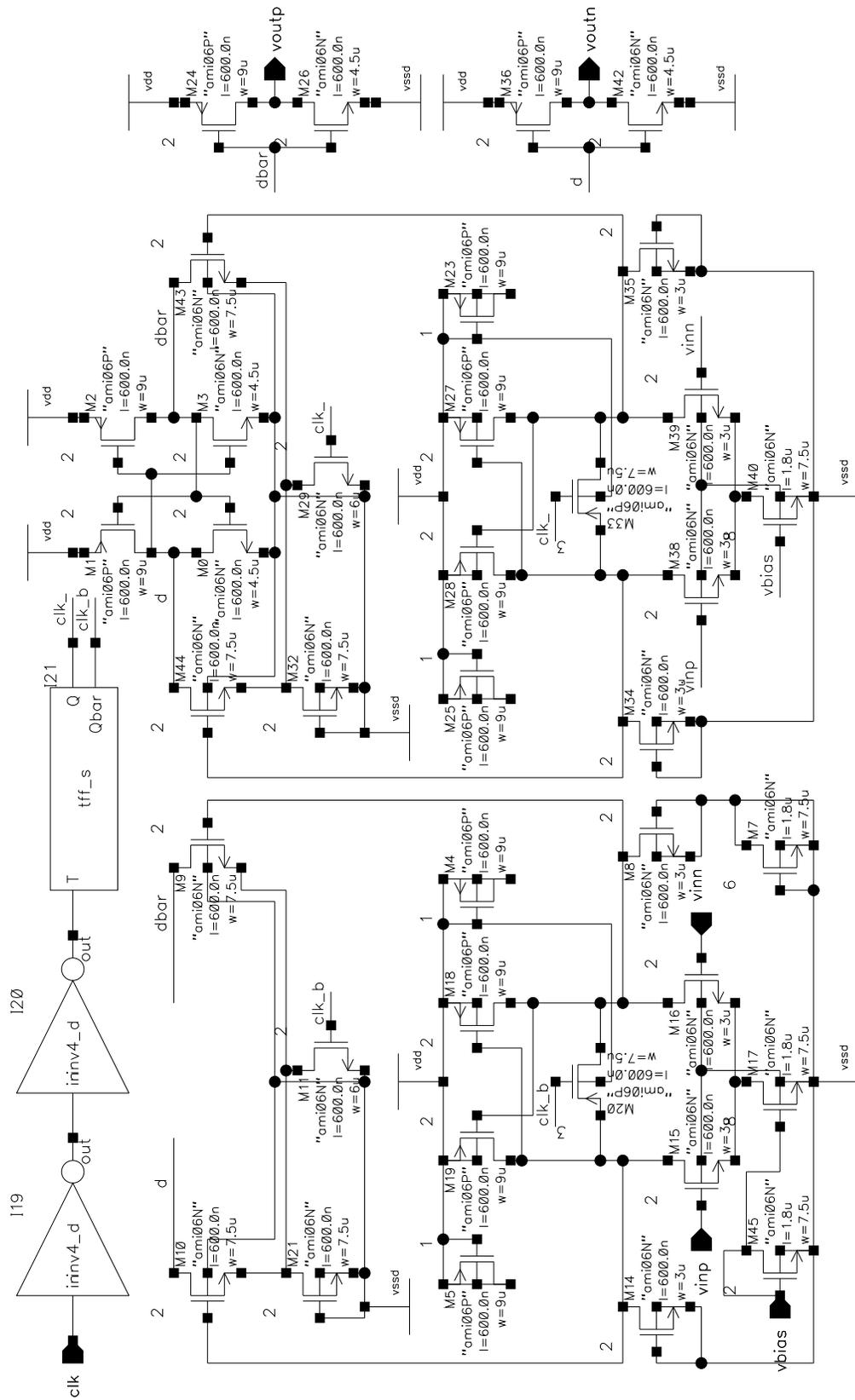
Figure A.2 Schematic of the dual-phase comparator.
