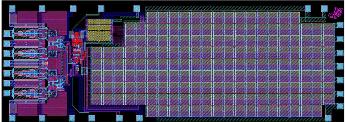
Figure 3.4 Partial die photo of delta-modulated supply circuit.
