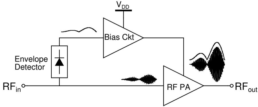
Figure 2.4 Block diagram of an ET PA.
