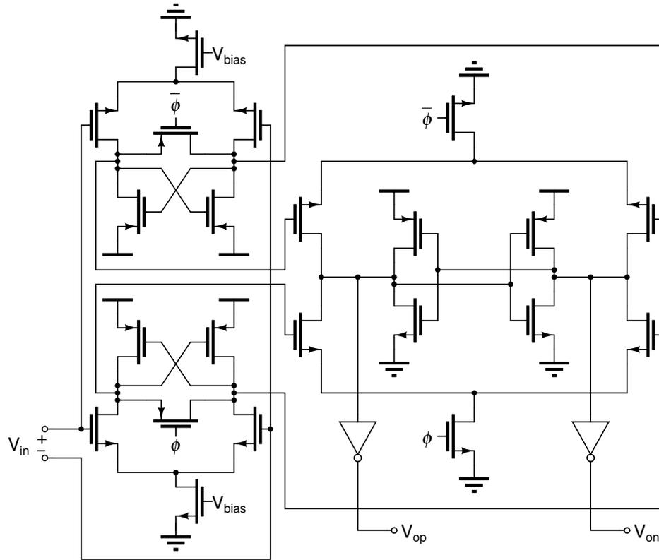
Figure 3.9 Synchronous comparator with low delay.
