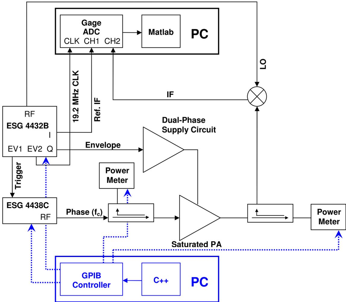
Figure 4.13 AM-AM, AM-PM, and EVM measurement setup.
