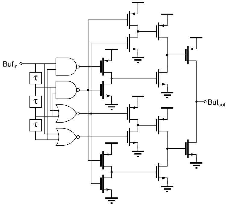
Figure 3.8 Tree-like buffer structure for reduced power loss.
