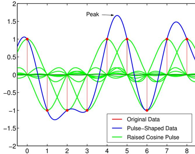
Figure 4.25 Binary data pulse-shaped with raised cosine filter.
