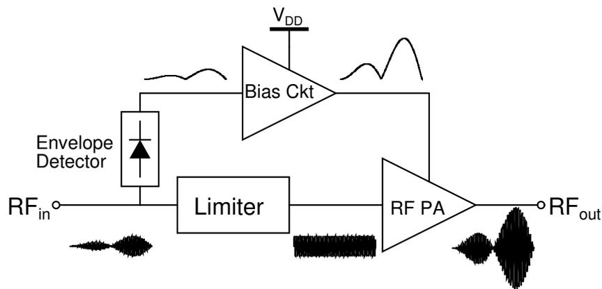
Figure 2.3 Block diagram of a basic EER PA.
