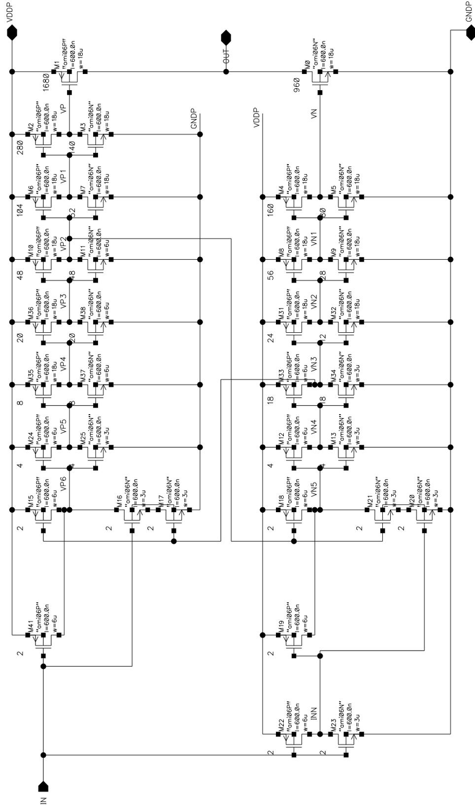
Figure B.8 Schematic of the switch and driver.
