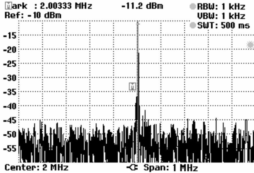
Figure 3.13 Measured spectrum of dynamic supply circuit with an 18  $\Omega$  load.
