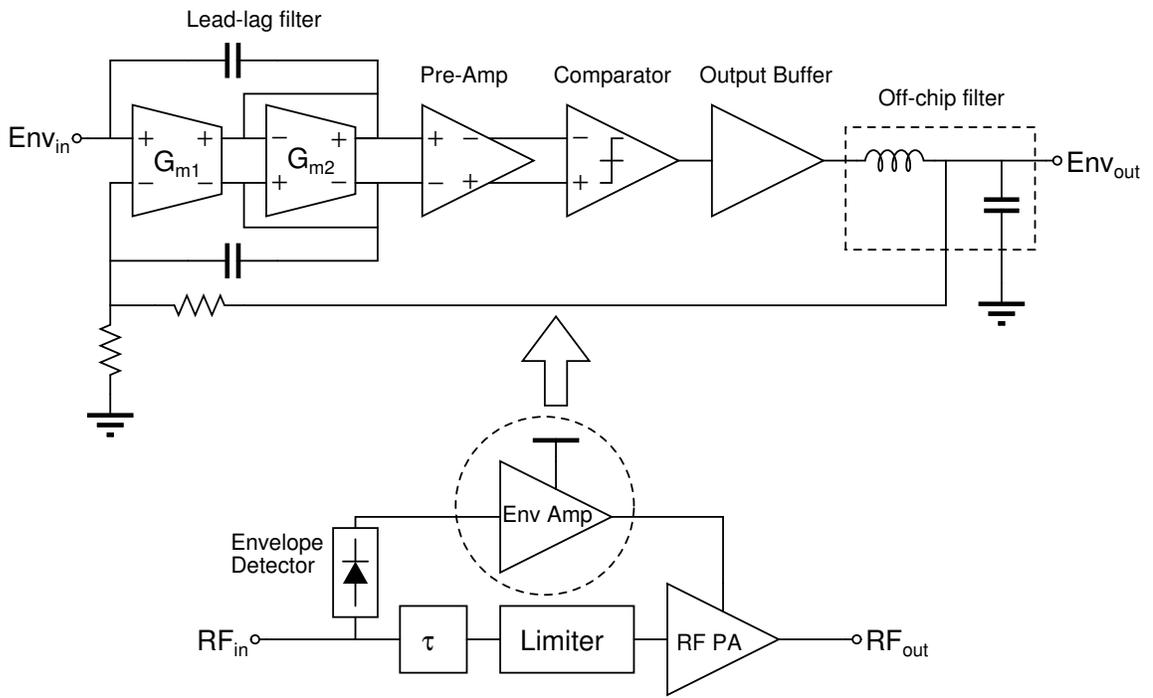
Figure 3.2 Block diagram of the dynamic supply circuit.
