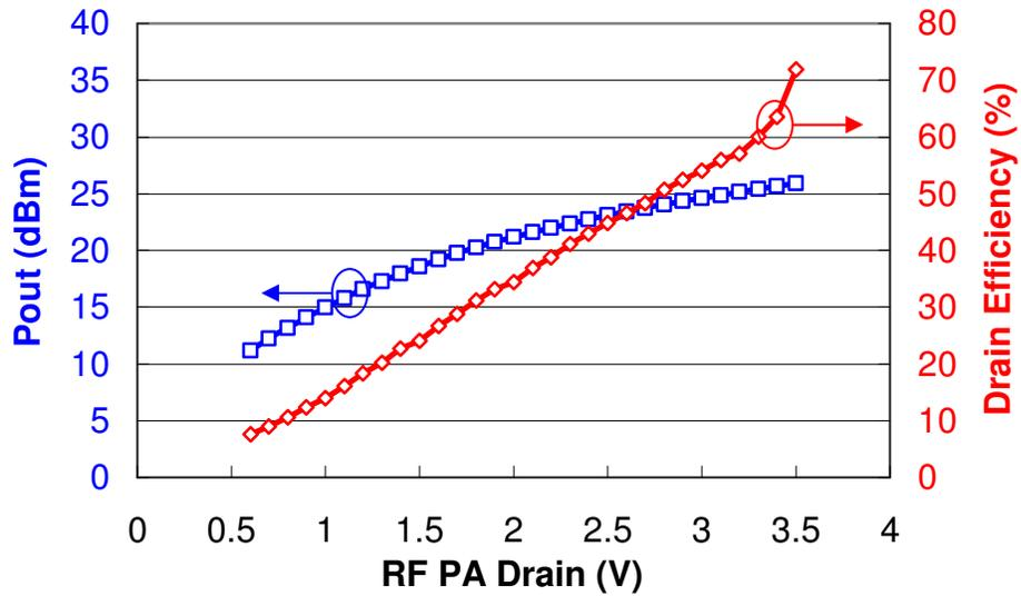
(b) Output power and drain efficiency
