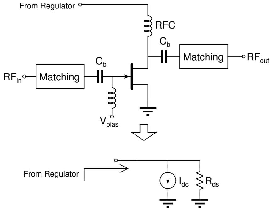
Figure 2.2 PA as a load to the regulator.
