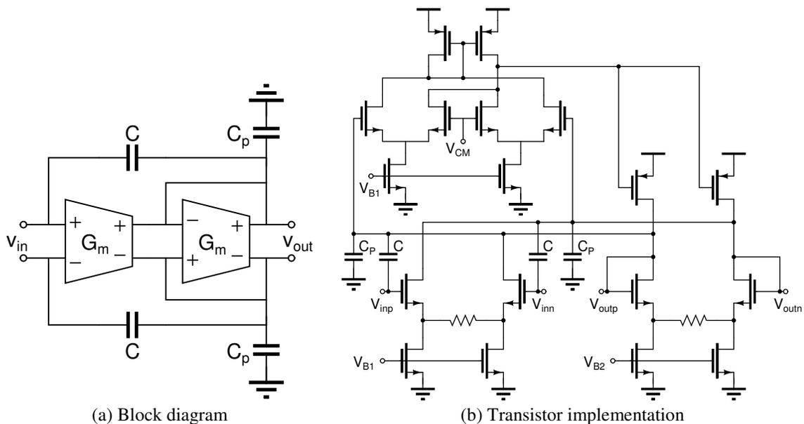
Figure 3.10 Implementation of lead-lag filter for phase compensation.
